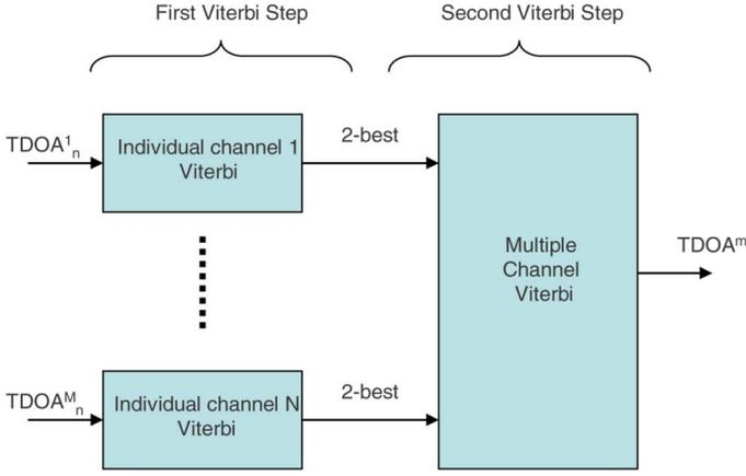
Fig. 2. Weighted-delay&sum double-Viterbi delays selection.
