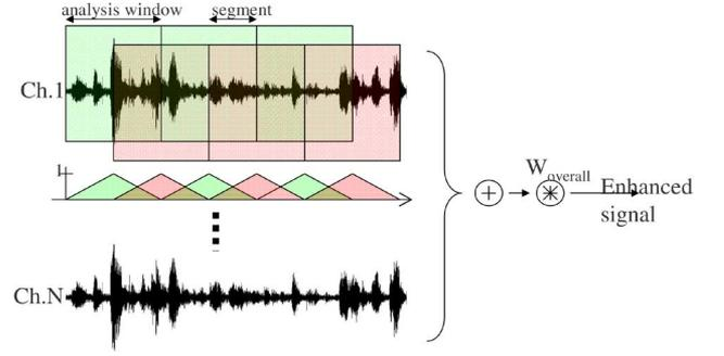
Fig. 4. Multichannel delayed-signal sum using a triangular window.
